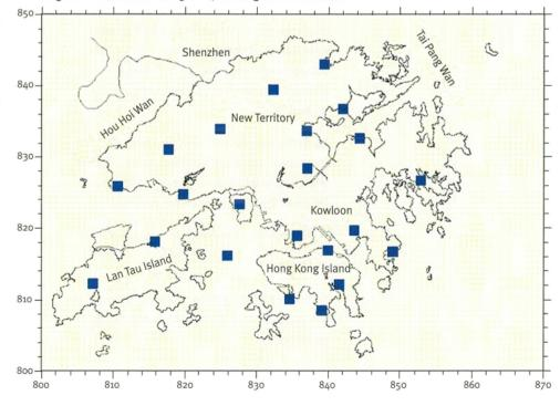
evaluated by comparing the geoid heights at these stations derived from the model NModel with that derived from GPS/Leveling  $N^{\rm obs}$  in absolute or relative sense, i.e.
