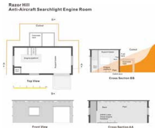
**Figure 86:** Different aspect views of the AASL Engine Room.
